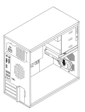
Figure 36. Installing a new internal speaker
